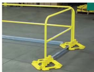
At each start or stopping point of leading edge railing run, install a 5' railing at 90 degrees from edge. Form "U" shape.
