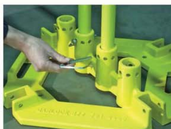
Insert securing pin to lock railing and base together.
